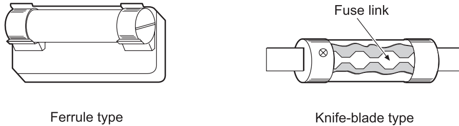
Figure 2—Ferrule type and knife-blade type cartridge fuses
