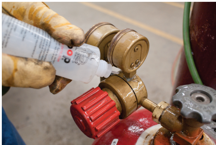
Figure 3—Apply a Soapy Solution to Locate Leaks
