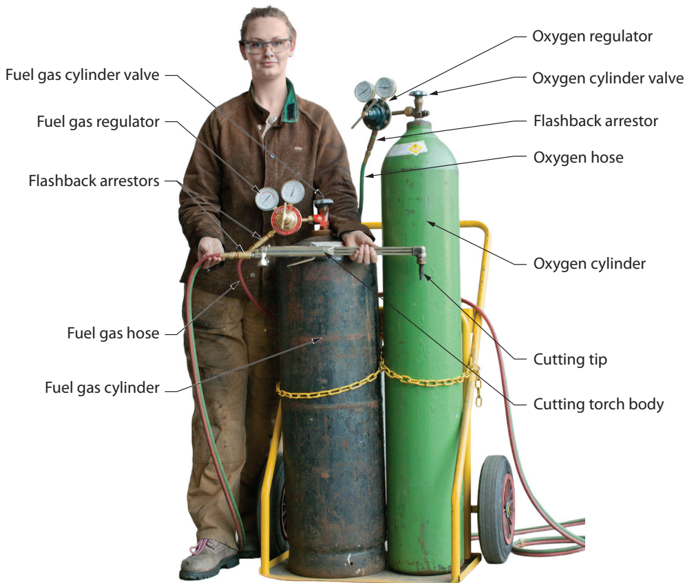
Figure 1—Portable Oxy-Acetylene Setup
