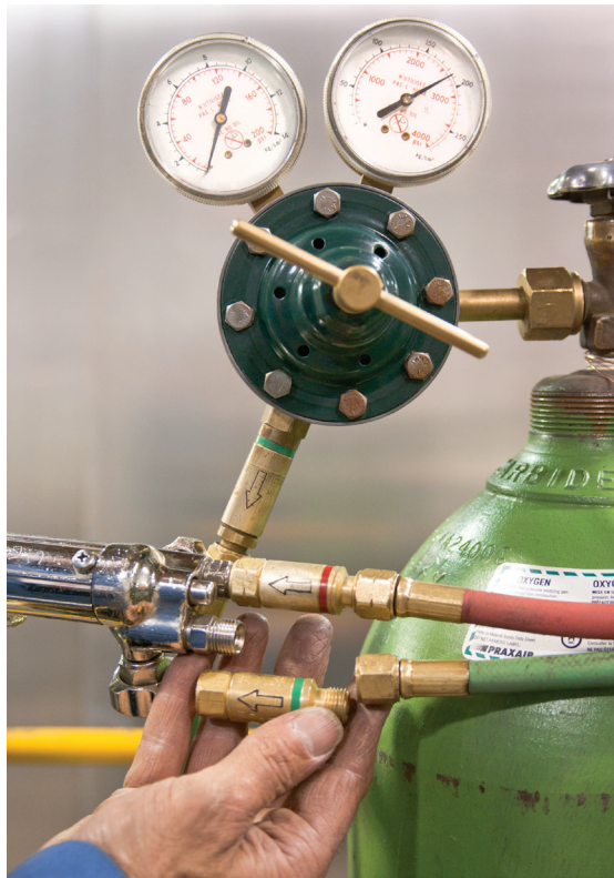
Figure 1—Oxygen Valve Controls Oxygen to Cutting Lever and Preheat Valve
