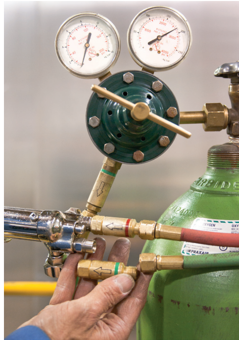
Figure 2—Installation of RFCVs
