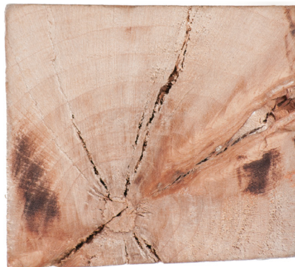
Figure 2 – Checks along the rays are called “pith shakes,” “heart shakes,” and “star shakes”
