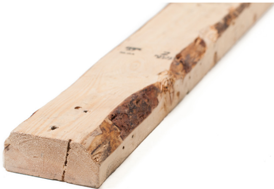
Figure 8 – Piece of lumber with wane
