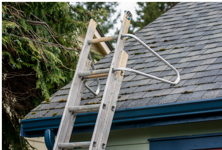
Figure 7 —Ladder standoff stopping the ladder from bearing against the eavestrough
