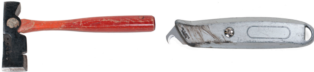
Figure 6— Roofer's hatchet and a roofer's knife
