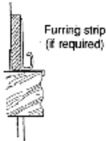
Figure 24—Inverted furring strip above window
